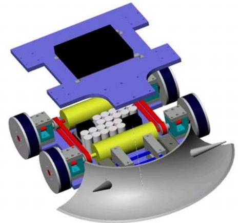
*Too much overhang (remember Saint-Venant!). Consider the use of an outrigger bearing, or mount the wheel on a properly supported shaft and drive the shaft with the motor using a coupling*
