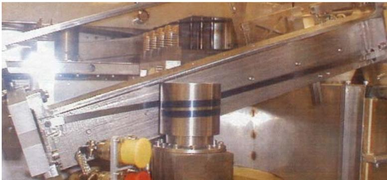
Should this metal belt driven axis be at this angle? NO, it was the software (honest) that made the vertical axis plunge while the metal belt driven horizontal axis was still extended...
