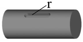
Corner r<br>Width b<br>Depth t | $\sigma = \frac{K_t 32M}{\pi D^3}$                     | $K_t = 1 + \frac{(r/d)^{-0.66}}{11.14}$<br>B=D/4, t=D/8                    |
