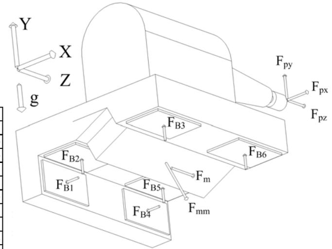
**Analysis (physics in words)** The magnet attraction force is 5x greater than the motor force, so it can be positioned at an angle such that even preload is applied to all the bearings. As long as the magnet attraction net vertical and horizontal force are proportional to the bearing areas and is applied through the effective centers of the bearings, they will be evenly loaded without any applied moments.
